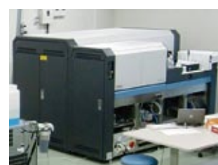
Double-focusing high precision ICP multi-collector mass spectrometer
