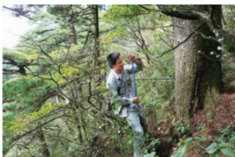
Photo 1 Collection of a tree-ring core from a pine tree
