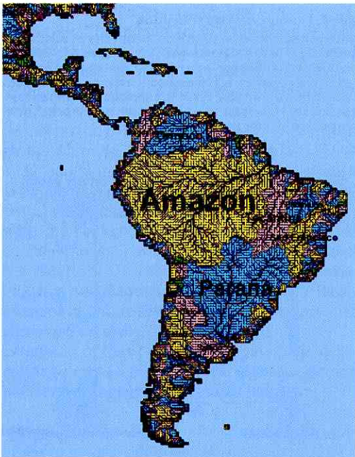
▲ Figure 1 Total Runoff Integrating Pathways (TRIP): Section in South America; The whole land on the Earth is covered with 0.5 degree longitude and latitude meshes and flow direction from each mesh is given. TRIP is coupled with land surface hydrological models and used to estimate the global potential water resources.
