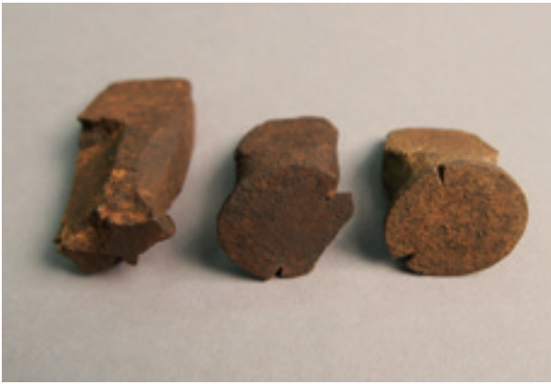
Photo 6. Comparison of mameya heads. Left: Greatly damaged mameya . Center: Partly damaged mameya . Right: Normally worn mameya .
