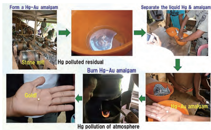
Figure 1 The Hg amalgamation process for getting gold in ASGM
