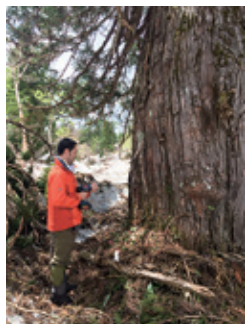
Photo 1 Sampling of a tree ring core from a living tree using an increment borer
