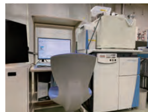
Isotope Ratio Mass Spectrometer connected with Elemental Analyzer (EA-IRMS)
