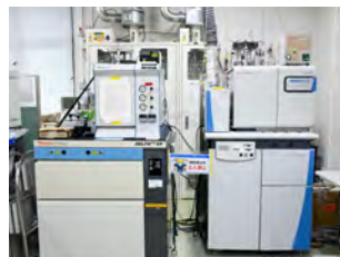
Isotope Ratio Mass Spectrometer connected with High-Temperature Conversion Elemental Analyzer (TC/EA-IRMS)
