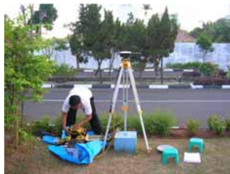
Fig. 9 GPS survey at Kunigung benchmark. We selected one of reference station for absolute gravity measurement.
