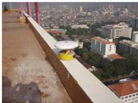
Fig. 7 GPS reference station at Chulalongkorn University.
