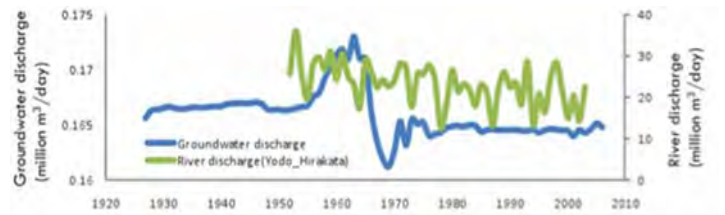
Figure 4. Simulated rates of fresh groundwater discharge compared with measured rate of surface water discharge to Osaka Bay
