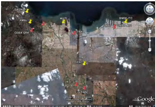
Fig. 10. Gravity points in Jakarta. The red pins show the absolute gravity points and the yellow pins show relative points.
