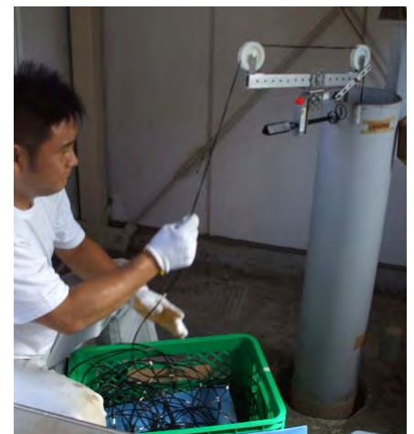
Fig. 3. Temperature measurement at a groundwater monitoring station
