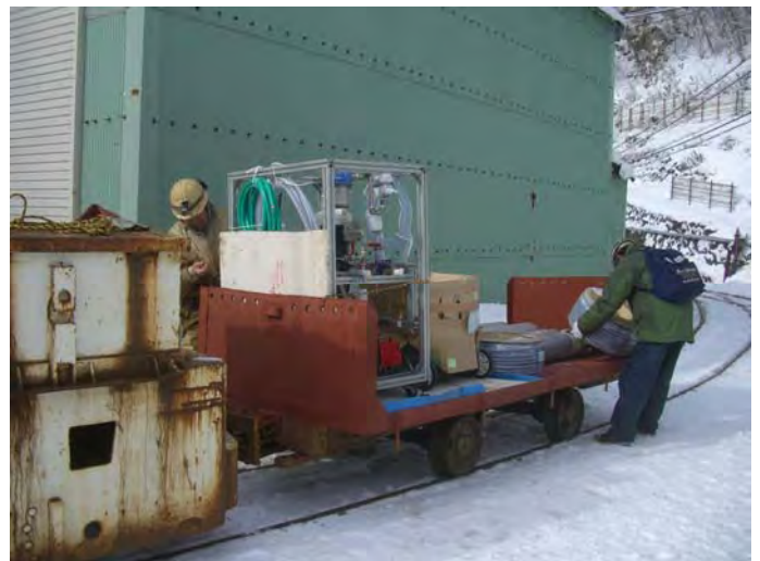
Fig.3 Battery rail car of the drift tunnel, its tunnel entrance and conveying sub-vehicle for the sampling tools.
