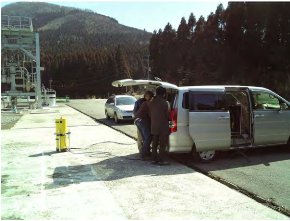
Fig. 8 Absolute gravity measurement at Takigami geothermal power plant.
