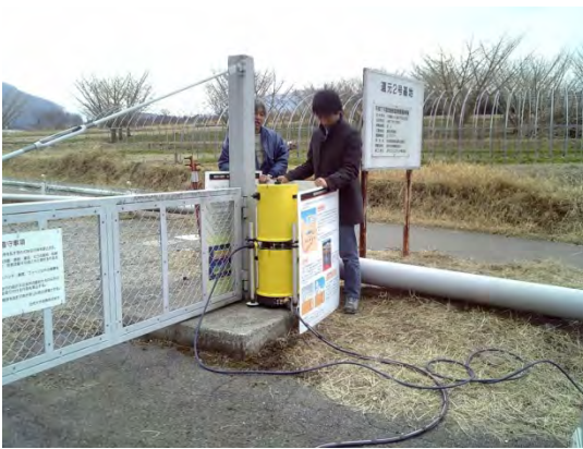
Fig. 10 The wind protection of the A10 absolute gravimeter.
