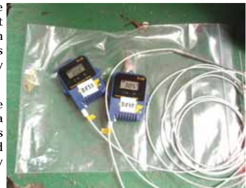
Fig.5. Temperature sensors and recorders used for soil temperature
