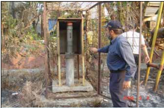
Fig.6. Bench mark for monitoring of land subsidence adjacent to a flowing well in Jakarta
