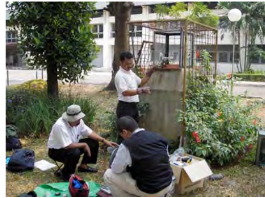
Fig. 1. Temperature profile measurement in a groundwater monitoring well in the Jakarta area.
