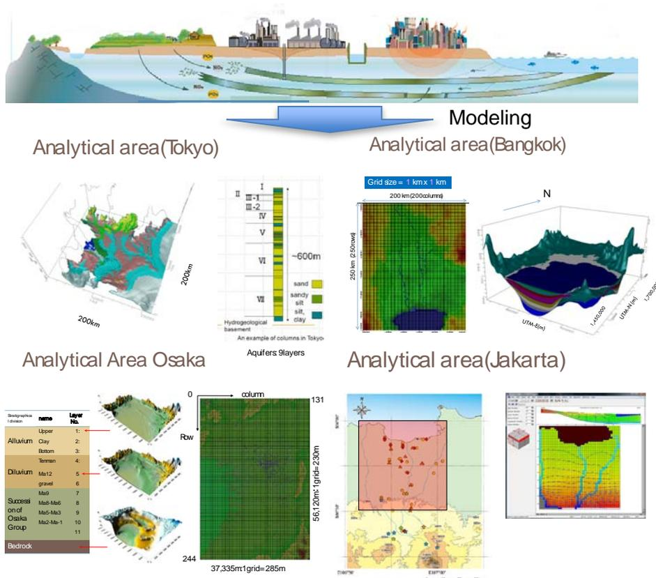
The Model Working Group (MWG) was formed to integrate the observation data from each area, collected by the Subsurface Environment Project. The groundwater flow in each city was analyzed using numerical simulation.
