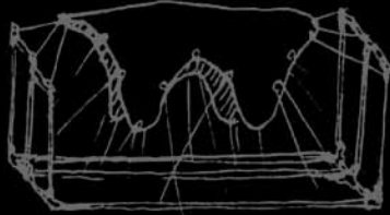
iron frame: l. 1000 X w. 2400 X ht. 1500 X φ15 wire: φ3
