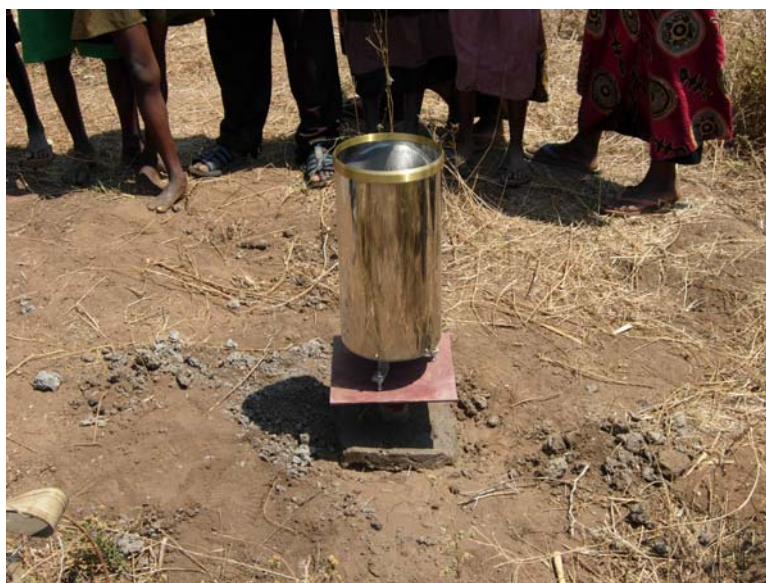
Fig. 2: Photograph of a rain gauge used in this study. The data logger is installed inside the gauge.
