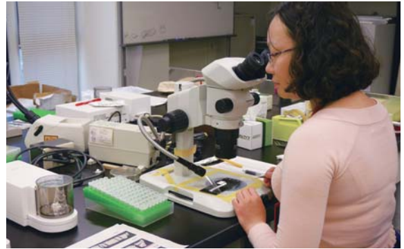
Photo 3 Separation of annual rings from wood cellulose in the laboratory
