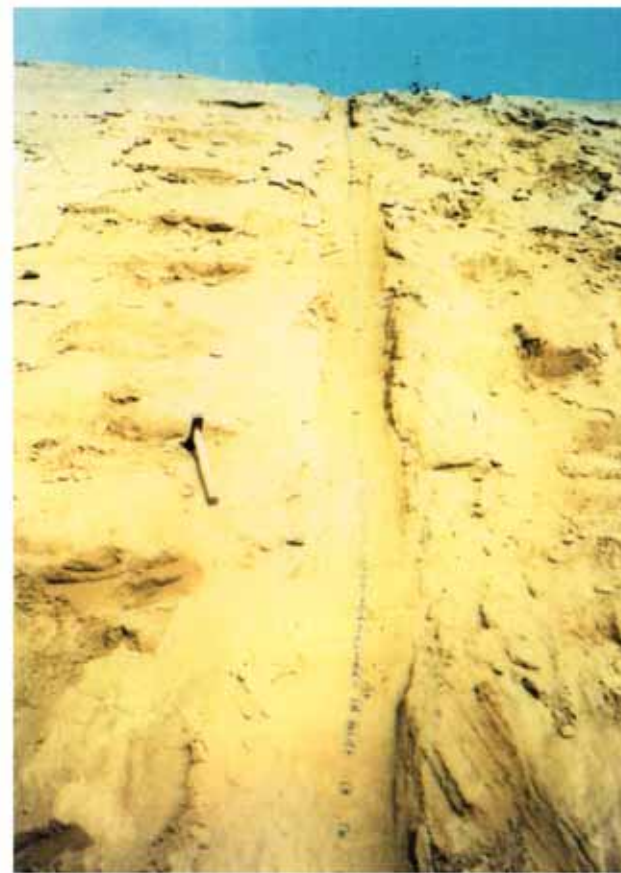
High resolution collecting samples of loess-paleosol sediments by using polycarbonate cubic samplers at Shajinpin section near Lanzhou
