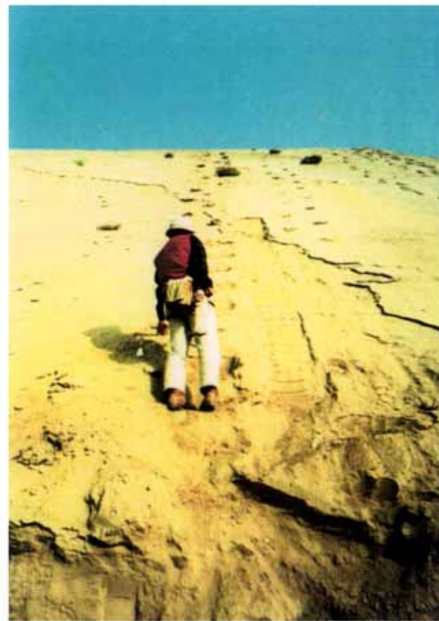
High resolution collecting samples of loess-paleosol sediments by using polycarbonate cubic samplers at Shajinpin section near Lanzhou
