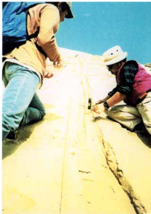
High resolution collecting samples of loess-paleosol sediments by using polycarbonate cubic samplers at Shajinpin section near Lanzhou
