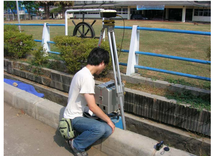
Photo 3: Gravity measurement using the relative gravimeter. Above the gravimeter the researcher is measuring the amount of ground subsidence using a GPS.
