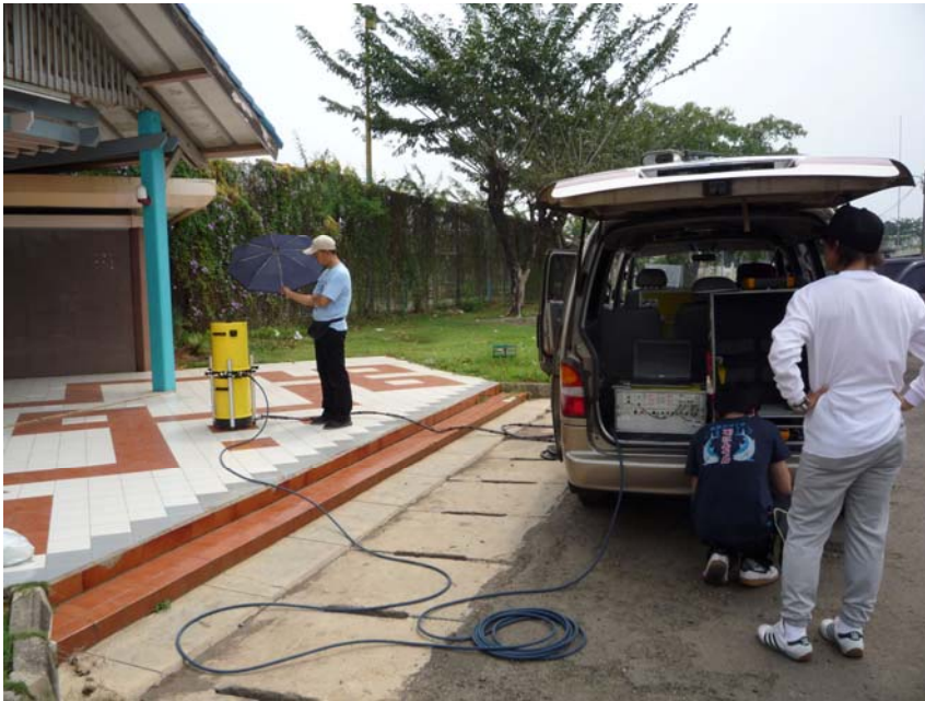
Photo 2: Gravity measurement using the absolute gravimeter. The controller in the vehicle carries out the measuring operation.
