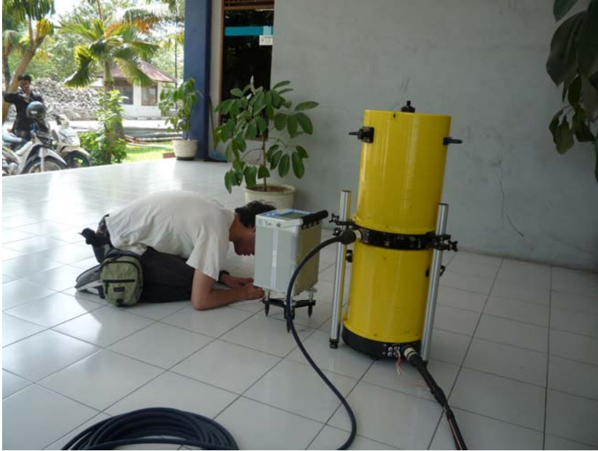
Photo 1: The relative gravimeter (left) and the absolute gravimeter (right).
