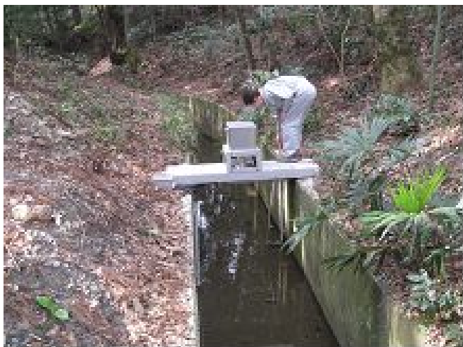
Monitoring water velocity and water level at water intake point from river
