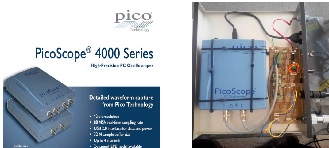
Figure 8. Analog to Digital Converter, PicoScope 4224.
