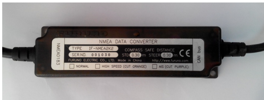
Figure 9. NMEA Data Converter (IF-NMEA2K2).
