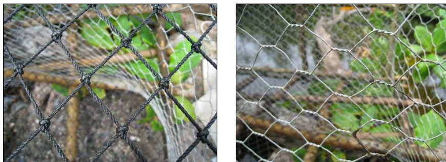
Fig. 3-4 Polyethylene netting (left) and wire netting (Right).
