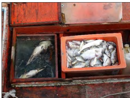
Fig. 3-10 The fish hold to keep live fish with seawater.
