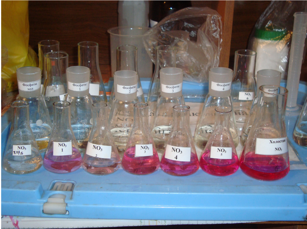
Fig. 3. Field Analysis of Nitrate Nitrogen (the Amur River at Nizhneleninskoe)
